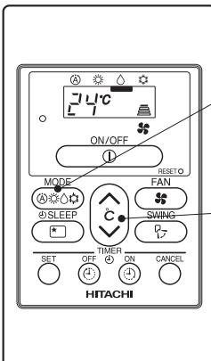
1 Press the MODE SELECTOR button so that the display indicates ◇ (DEHUMIDIFY).
