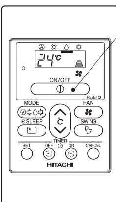
■ As the settings are stored in the memory in the remote controller, you only have to press the ① (START/STOP) button next time.
